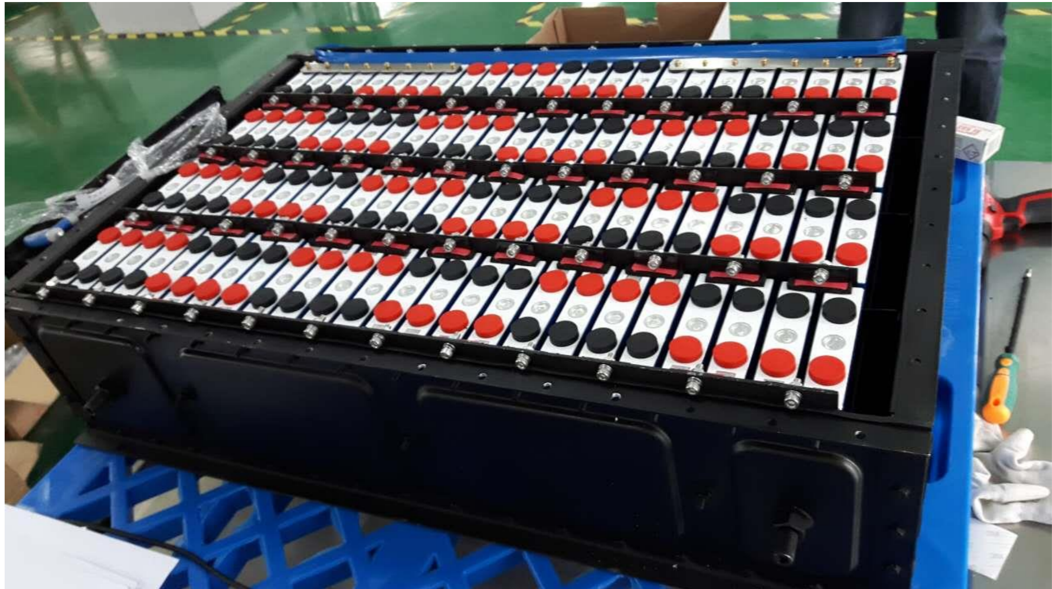
Standard C pack ( 1060 x 630 x 250 mm), with 96 pcs of 68 Ah (1.5 kg/cell) LFP cell, Capacity: 20.9 kWh, Total weight: 190.15 kg, Energy density: 110 Wh/kg
