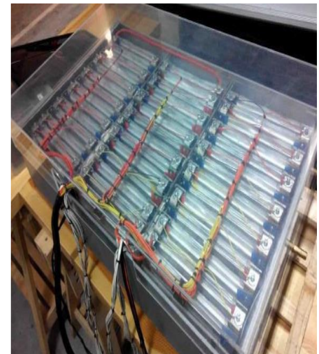
Battery Pack Assembled (8)
